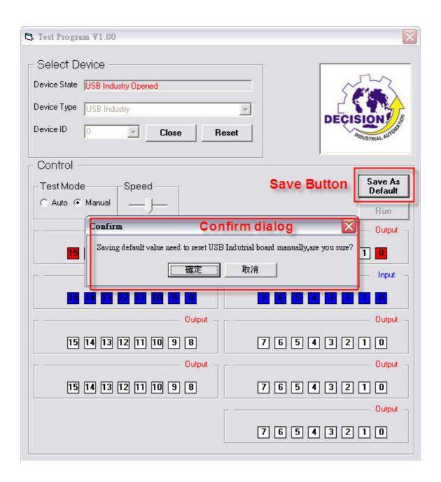
6. When finishing setting, please press the reset button on the board. And use this tool carefully due to init value you set will be loaded when power on, it may cause damage for its init state changed.
