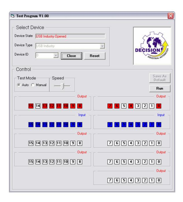
**4.** Switch into Manual mode , you can set init value on output port by clicking the output bit and init input/output setting of the port by clicking the Output / Input tag.
